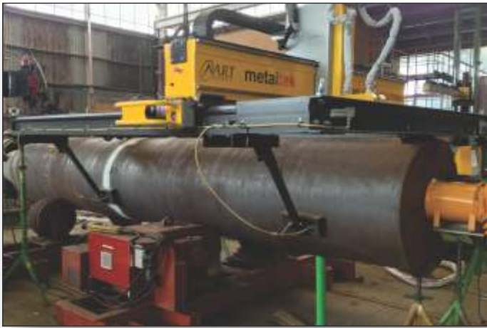
Vacuum or magnetic arms grip the vessel wall for stability
