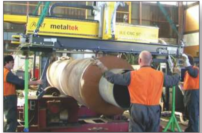
CNC machine is positioned onto the pressure vessel by crane
