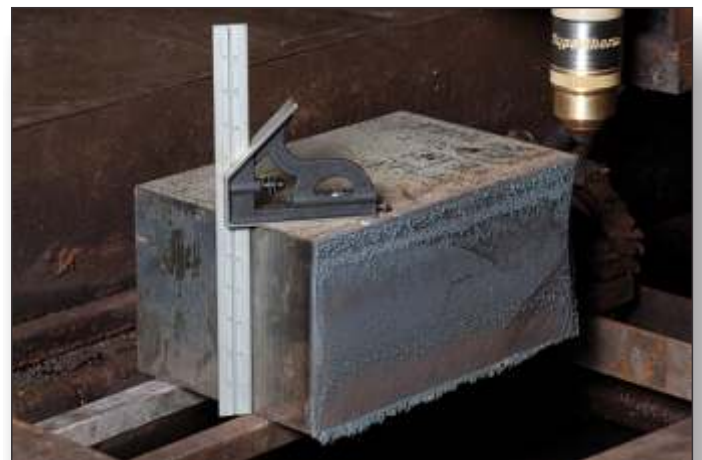
160mm capacity in stainless steel allows 45° bevels in 100mm walls
