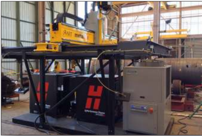
Machine is stored & transported on platform along with plasma units
