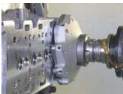
■ Rotating head for machining on vertical or overhead surfaces
