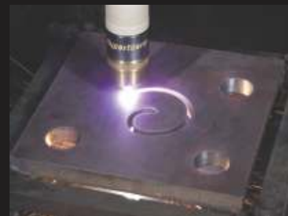
■ High definition plasma cuts steel, stainless and aluminium
