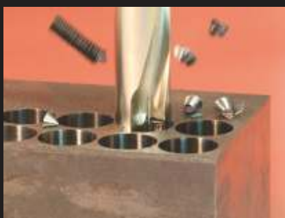
■ Drilling using indexable insert drills.
