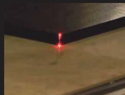
■ Laser digitising allows tracing of existing parts for duplication.
