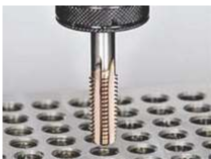
■ Rigid tapping using conventional thread taps
