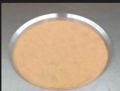
■ Bevelling/chamfering using angled milling cutters.
