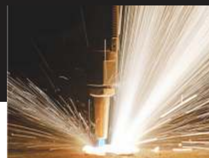
■ Oxy-acetylene torches enable accurate cutting of thick plate.
