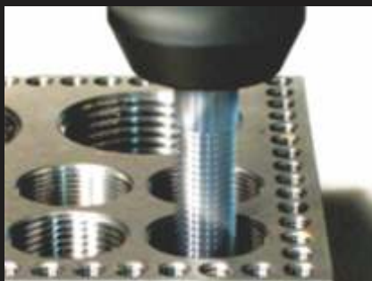
■ Thread milling allows treads of any diameter and pitch to be cut.
