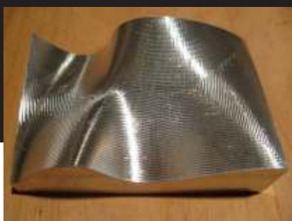
■ Contoured surfacing using ball nose cutters.
