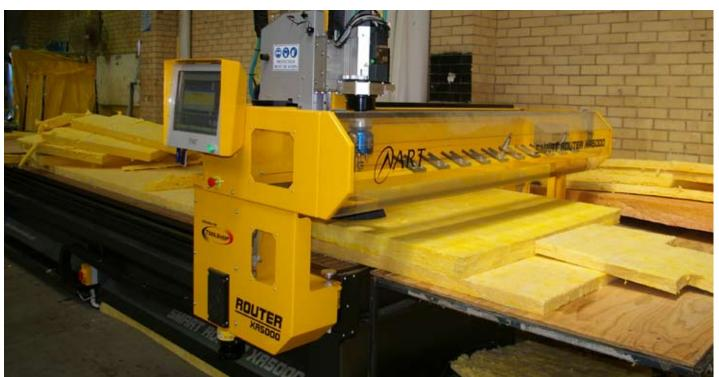
While Apex Insulation predominantly cuts fibreglass insulation with a reciprocating knife on the machine, the additional fourth axis on the CNC router offers many special tools designed for insulation material and duct board cutting including variable angled knives or steered pizza cutter wheels for creasing and cutting a variety of materials.
