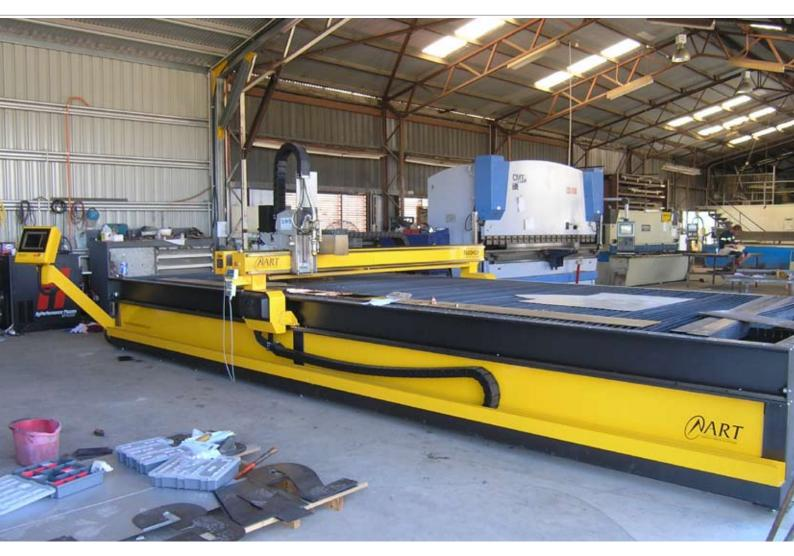
ART's HDP plasma cutter delivers economic processing of high-standard cut components with an edge quality that is comparable with laser cutting; a feature which gives Riggs Sheetmetal the decisive competitive edge over its competitors.
