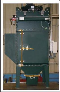
Industrial quality fume extractors are supplied for optimum health and safety purposes. Large metal ducting provides less drag and improves efficiency. The Extraction and filtration system works in conjunction with the downdraft extraction deck to remove most of the fumes and dust from your workshop environment.
