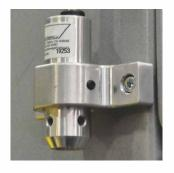
along the bottom or side of the plate. This allows the controller to rotate the job to fit material in the event that is not placed squarely on the cutting deck. The controller activates the laser and calculates the offset to the torch automatically.
